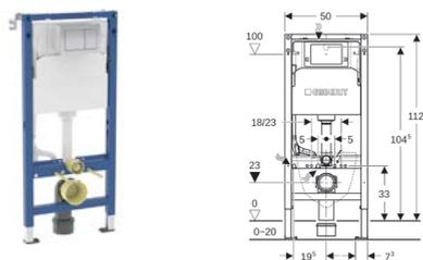
**Geberit Duofix element for wall-hung WC, 112cm, with Alpha concealed cistern 12cm, 6/3 litres with square flush plate**
