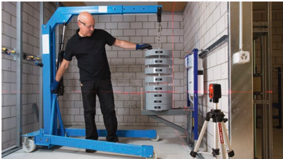
Geberit Duofix is tested for strength and durability. Six metal plates weighing in excess of 400kg (63 stone) are loaded on to a support acting as the WC.
