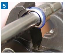
Must use correctly sized jaw/collar. Fittings must be aligned correctly in jaw/collar. Ensure insertion depth is met before pressing!
