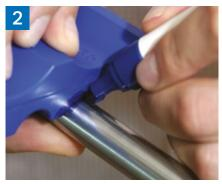
To ensure the pipe is fully inserted before pressing. Gives visual security. This is very important!
